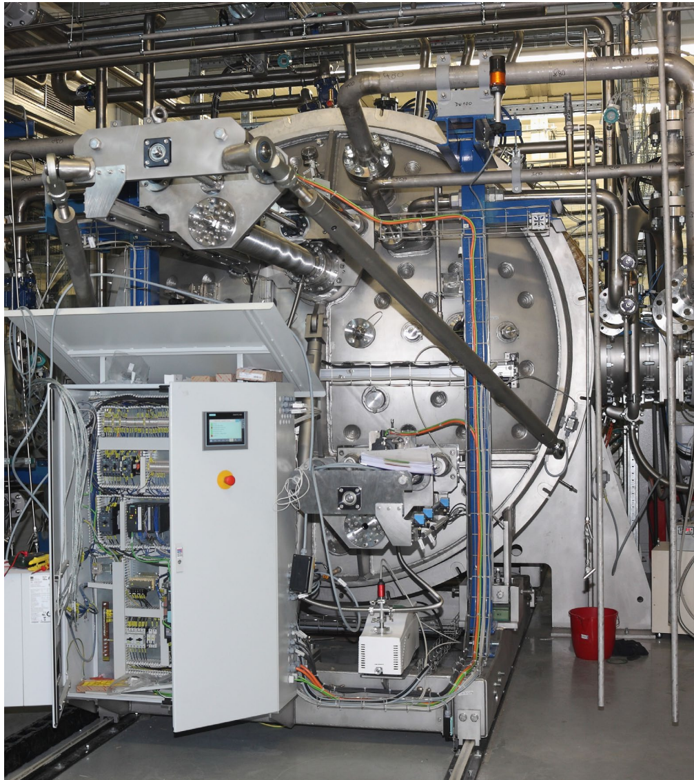
Testing Vacuum Unit HELCZA F4E / ITER High Heat Flux Test Facility for Testing of ITER EU First Wall Components
